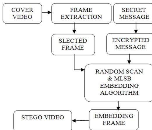
**Fig. 2 Experimental setup of Video Steganography**
