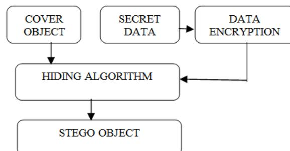
Fig. 1 Block Diagram of Steganography
